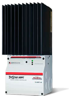
Figure 1. Morningstar MT MPPT controller The MT MPPT provides several communication options. The MT MPPT uses a proprietary protocol for the MeterBus network and the non-proprietary open standard MODBUS RTU and MODBUS TCP protocols for RS-232, EIA-485,
