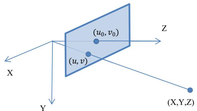
Figure 1. The camera coordinate system and the projection of a 3D point  $(X, Y, Z)$  in the image plane
