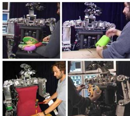
Fig. 1. The experimental platform. The humanoid robot Cog is equipped with cameras in an active vision head, a microphone array across the torso and two robotic arms. Some typical learning scenarios (from left to right, top to bottom) a human shows a book to Cog; a human describes the shape of an object to the robot; a repetitive action (hammering) is demonstrated to the robot; a human waves a yellow car to create a salient stimulus on Cog’s attentional system.
